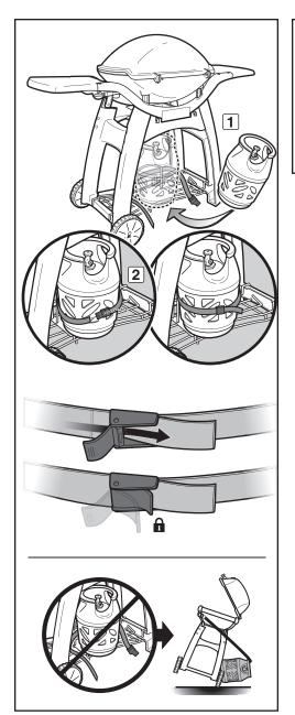
Maximum LPG cylinder capacity when INSTALLED ON CART under the barbecue is 6 kg.
